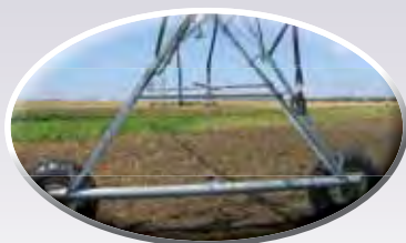
Towable 1 tower water driven centre pivot wets up to 3,8 ha
